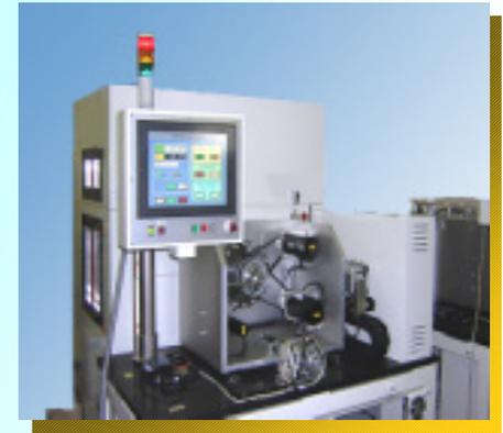
This equipments gives the tray-supplied MEMS a characteristic inspection at three temperature areas - high, normal, low - at any angle. MENS are put in each tray according to the result of the inspection.
