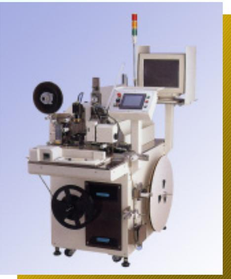
This equipment inserts the electronic part into the emboss carrier tape with stick supply. It is the standard image processing device that inspects the size and appearance of the part and does cover tape sealing and reel winding of only good items automatically.
