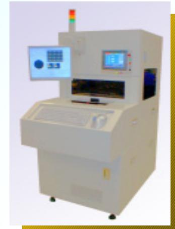
This equipment has composite lightings and high resolution colored camera. It inspects the appearance of the chip with defects at high speed and accuracy.
